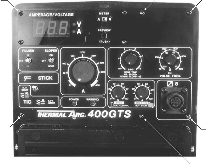
Figure 23. Front panel circuit board retaining screws (shown in GTS model)
