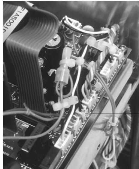
Figure 36. Power control assembly - thermal sensor (shown in GMS model)
