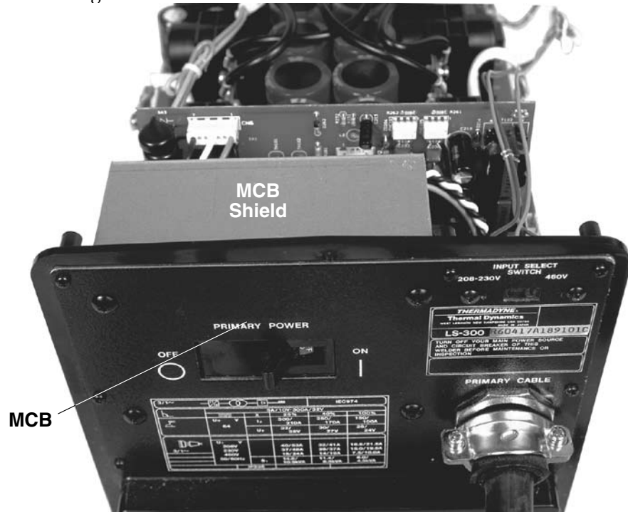
Figure 13. MAIN CIRCUIT BREAKER (shown in GMS model)
