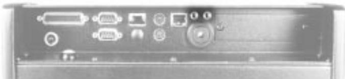
*Figure 15. Audio Input/Output*
