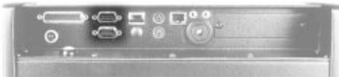
*Figure 11. Serial Port (DB9) Connectors*
